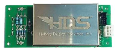
The HDS Voltage Sense Board (VSB) consists of a full-featured, isolation amplifier that measures voltage readings up to 1000V DC, and provides an analog 0-5V signal output. The VSB provides isolation between signal and power for safe operation.
